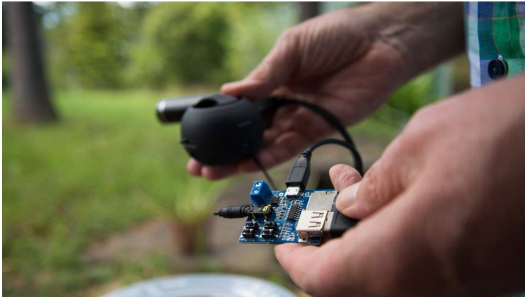
The male mosquito lure is made from cheap and simple components including a circuit board that acts as an MP3 player, a battery pack and a speaker, but it is highly effective at attracting male mosquitoes into the trap. ABC Far North: Mark Rigby
